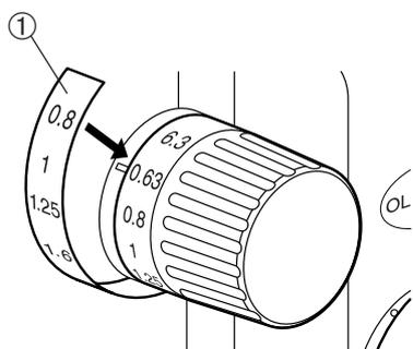
Ⓞ The DFPLAPO1.25X objective is provided with a sticker that indicates a set of total magnifications available\* during observation.
