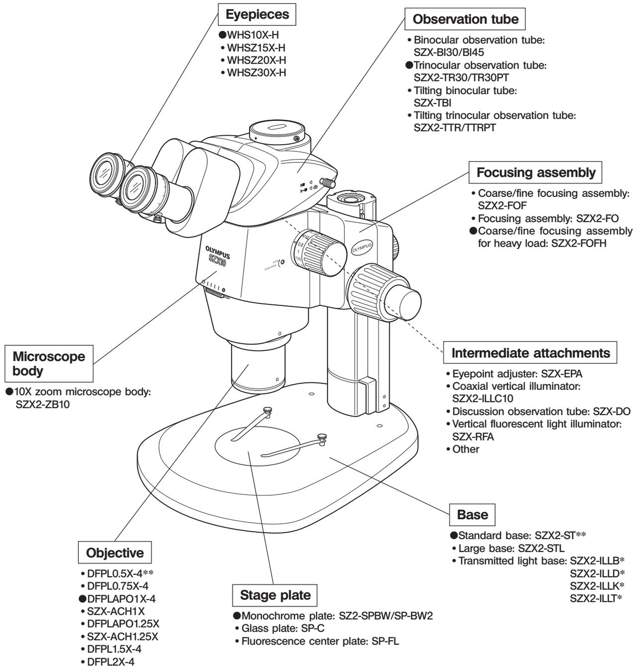
\*\* The standard base (SZX2-ST) requires use of the optional auxiliary pillar (SZH-P400) and optional drop prevention collar (SZX-R). The large base (SZX2-STL) comes with the auxiliary pillar (SZH-P400) mounted as standard. This enables the large base to be used as is. However, be sure to use the drop prevention collar (SZX-R) in combination.
