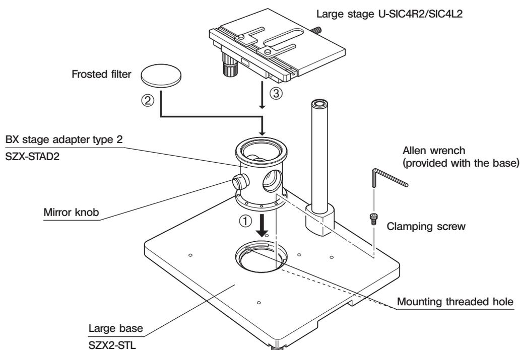
★ For simplified transmitted light observation, place the mirror knob on the front and use a frosted filter.
